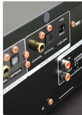
Can be used as a D/A converter with 3 digital inputs (coaxial, optical, USB type B)
