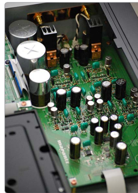
Analog audio circuitry featuring Marantz's unique HDAM technology
