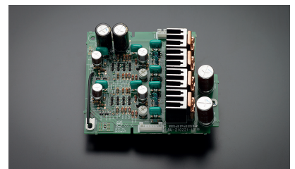
Fully discrete headphone amplifier
