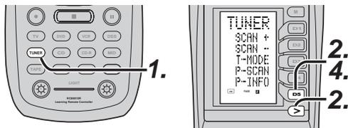
1. Press the Tuner button on the remote controller twice within two seconds to switch to the TUNER function.
