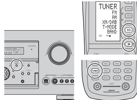
1. Press the **>** button on the remote controller to display Page 2.
