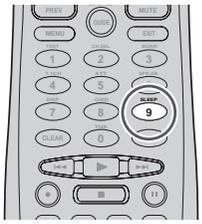
To program this unit for automatic standby, press the **SLEEP** button on the remote controller. Each press of the button will increase the time before shut down in the following sequence.
