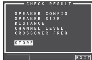
Place the cursor on **STORE** and press the **OK/ENTER** button to store all parameters including the equalizer parameters in memory. If not wanting to store the calculation results in memory, place the cursor on **EXIT** and press
