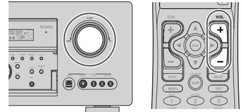
Adjust the volume to a comfortable level using the **VOLUME** control knob on the front panel or **VOLUME ▲ / ▼** buttons on the remote controller.
