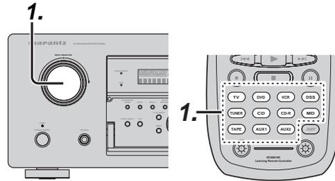
1. Select the input source to record by turning the **INPUT FUNCTION SELECTOR** knob on the front panel or simply press the input selector buttons on the remote controller.
