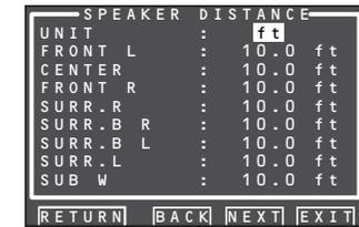
Use this menu to specify the distance of each speaker's position from the listening position. The delay time is automatically calculated according to these distances.
