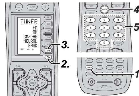
1. To select tuner, Press the **TUNER** button twice within two seconds on the remote controller.
