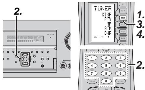
1. Press the **PTY** button in the **TUNER MODE** on the remote controller. The current station's PTY will be displayed, or the currently selected PTY group will be displayed in blinking if no station or RBDS data is present.
