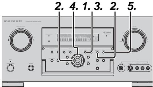
1. To select FM, press the **BAND** button on the front panel.
