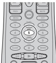
If the selected analog audio input signal is greater than the capable level of internal processing, the **"PEAK"** indicator will light up on the front display. If this happens, you should press the **ATT** button on the remote controller.
