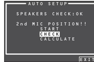
Here, to view the results of the detection check, select "CHECK" with the ▲/▼ cursor buttons and press the OK/ENTER button. The results will be displayed.
