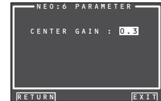
4. Set the CENTER GAIN level between 0.0 and 1.0 in 0.1 level increments with the **◀** or **▶** cursor buttons.
