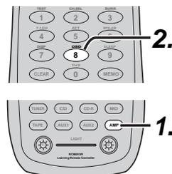
1. Press the **AMP** button on the remote controller.
