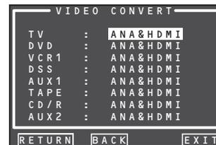
3. Select "FUNCTION" with the ▲ / ▼ cursor buttons and set the video conversion mode with the ◀ / ▶ cursor buttons
