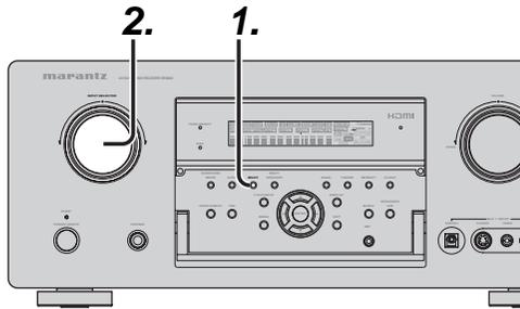
1. Pressing the **MULTI** button on the unit one time accesses the MULTI ROOM A settings. Pressing it two times accesses the MULTI ROOM B settings. Then, pressing it a third time turns the multiroom feature off. (The SR7002 does not have a MULTI ROOM B setting.)
