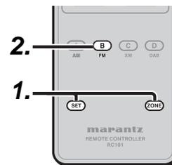
1. Press **SET** button and **ZONE** button until the SEND indicator blinks twice. Then backlight flashes.
