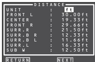
\* The units can be changed by moving the cursor to [ft] of UNIT and pressing ◀/▶ the cursor buttons. Each time a ◀/▶ cursor button is pressed, the units alternate between [ft] (feet) and [m] (meters).
