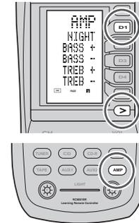
1. To select this mode, press the **AMP** button on the remote controller, and then press the **>** button until **PAGE3** is displayed.
