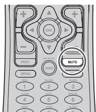
To temporarily silence all speaker outputs such as when interrupted by a phone call, press the **MUTE** button on the remote controller. This will interrupt the output to all speakers and the head-phone jack, but it will not affect any recording or dubbing that may be in progress. When the system is muted, the display will show "MUTE". Press the **MUTE** button again to return to normal operation.
