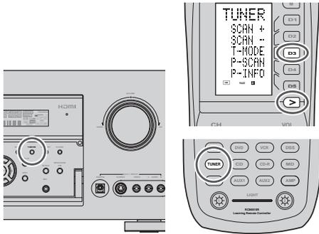
In TUNER mode, press the **T-MODE** button on the remote controller to switch between AUTO STEREO and monaural sound.
