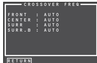
\* AUTO is displayed to indicate that the speaker size and crossover frequency results were automatically measured.
