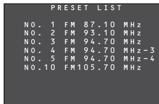
In the list of preset channels above, preset numbers 4 and 5 are the multicast channels for preset number 3.
