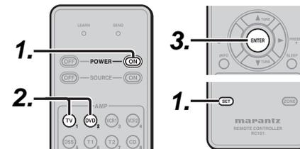
1. Press **SET** button and **POWER ON** button until the SEND indicator blinks twice. Then backlight flashes.
