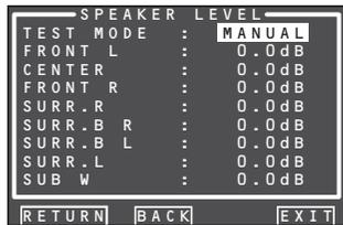
Here you can set the volume for each speaker so that they are all heard by the listener at the same level. We recommend holding a dB SPL (Sound Pressure Level) meter at the listening position, at arms length, and pointing straight up at the ceiling, adjust the level of each speaker in turn until it reads 75dB SPL when the meter is set to "C" weighting and Slow response.
