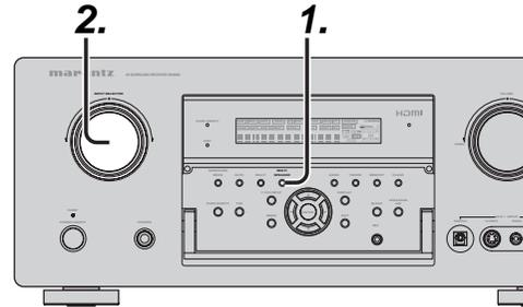
1. Pressing the **MULTI SPEAKER** button on the unit one time accesses the MULTI SPEAKER A settings. Pressing it two times accesses the MULTI SPEAKER B settings. Then, pressing it a third time turns the MULTI SPEAKER feature off. (The SR7002 does not have a MULTI SPEAKER B setting.)
