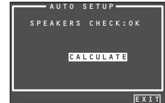
Select "CALCULATE" with the ▲/▼ cursor buttons and press the OK/ENTER button to calculate measurement results. During calculations, the following OSD appears on the display.
