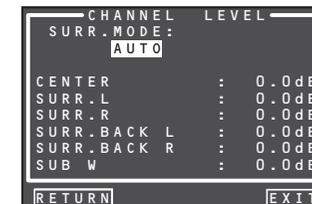
4. Select the desired menu item with the ▲ or ▼ cursor buttons, set the desired level with the ◀ or ▶ cursor buttons, and press the **OK/ENTER** button.
