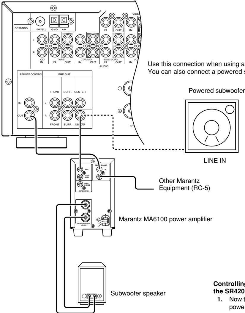
**Controlling the power ON/OFF of a power amplifier connected to the SR4200 through Marantz remote control**
